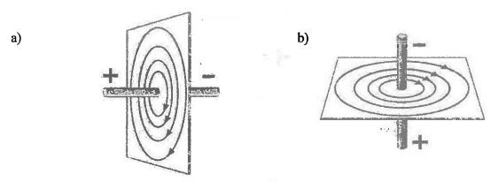
A) This field representation matthesthe right-hand rule. If the right thumb points to the negative direction the fingers point to the frelk direction.
