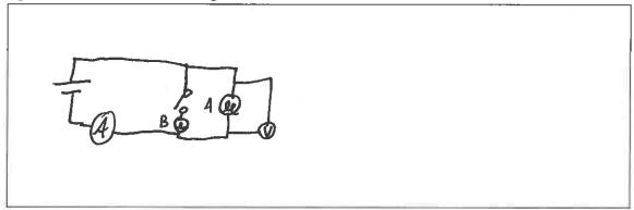
a power supply, two light bulbs connected in parallel, two switches, one that controls
