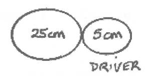
a) Does the driven gear rotate faster or slower than the driver?
