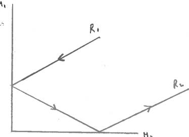
Light ray  $R_1\,\text{hits}\;M_1\,\text{and}$  is reflected. It hits  $M_2\,\text{and}$  is again reflected.
