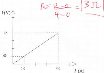
The following graph shows the variation in the current intensity, *I*, as a function of the potential difference (voltage), *V*, across a resistor.
