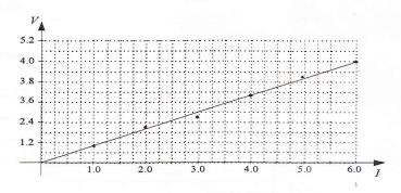
Calculate the resistance of this circuit element.
