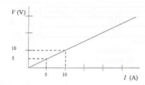
According to the graph, what is the resistance of the resistor?
