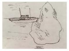
$$\begin{split} & m_{displaced \ water} ^*g = m_{iceberg} ^*g \\ & m_{displaced \ water} = m_{iceberg} \\ & V_{displaced \ water} ^*d_{water} = V_{iceberg} ^*d_{iceberg} \end{split}$$
