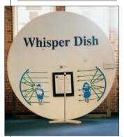
wHISPER DISHES are two parabolic dishes set up facing directly toward each other. A person listening at the focus of one dish is able to hear even the softest sound made at the focus of the other dish.
